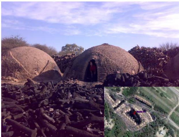
Figure 8. Charcoal ovens in the dry Chaco of Argentina. Poorly quantified and studied, these facilities and the whole charcoal production chain, represents the main productive energy output of the region, suggesting that these dry forest are already focused on “bioenergy” production. Our team is developing new tools to quantify their energy and charcoal output with the aid of remote sensors. We are also exploring the diversity of actors and contexts in which charcoal production takes place, including large multifamily systems associated with forest clearance operations (agricultural expansion) and small traditional single-oven systems run by one family, usually in association with livestock production.
